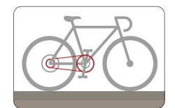
A cyclist can ride up a hill by using a small gear that is easier to pedal attached to a larger gear, which turns the back wheel slowly but with more force.
